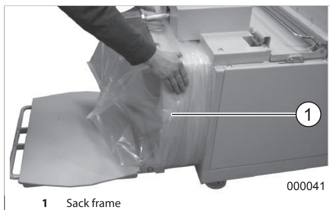
fig. 19 Installing a new plastic sack
